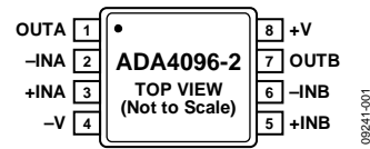
Figure 1. 8-Lead, MSOP (RM-8), ADA4096-2
